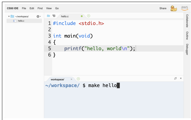
Figure 3: CS50’s first web-based programming environment, CS50 IDE, was ultimately built atop AWS Cloud9, backed by a Kubernetes cluster of Docker containers. Upon login, students were allocated a newly created container to which their own home directory was attached. Students could then write, debug, and execute code within that container via a web-based UI, complete with a code editor, file explorer, and terminal window, with AWS Cloud9’s default UI both simplified and enhanced for teaching and learning via the course’s own plugins.
